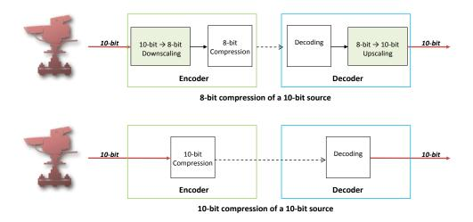
However, this is only a part of the story: encoding pictures using 10-bit processing always saves bandwidth compared to 8-bit processing, *whatever the source pixel bit depth*.
